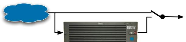
The DVStor can even be configured to start playout automatically upon detecting input loss.
