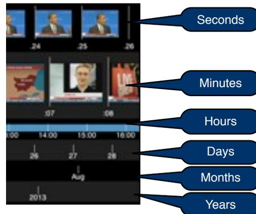
The main browser display is divided into six time bands which show from years all the way down to seconds, letting you quickly scroll to any point in time.
